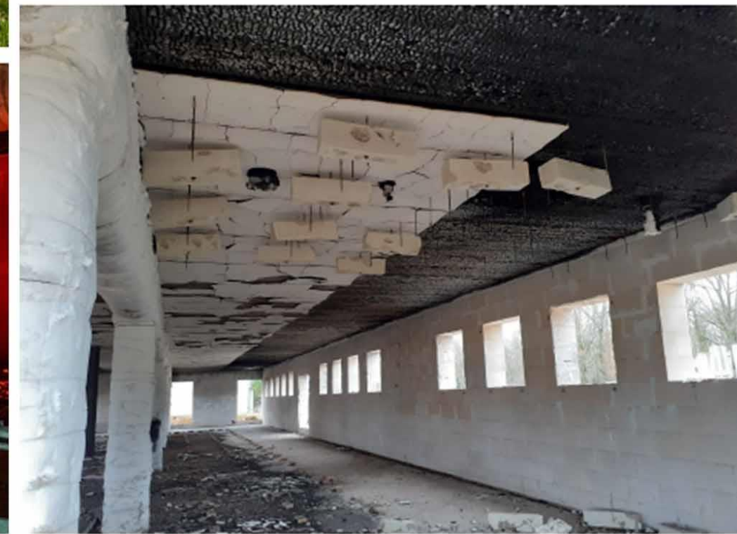
large-scale fire tests being conducted on timber compartments (ARUP, 2021)
