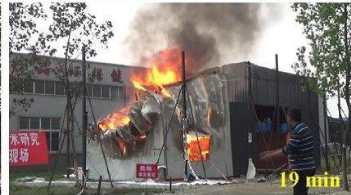
Fire testing of a steel structure in China
