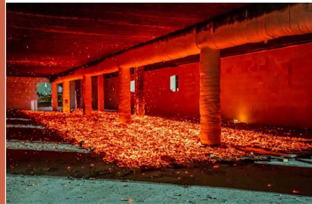
large-scale fire tests being conducted on timber compartments (ARUP, 2021)
