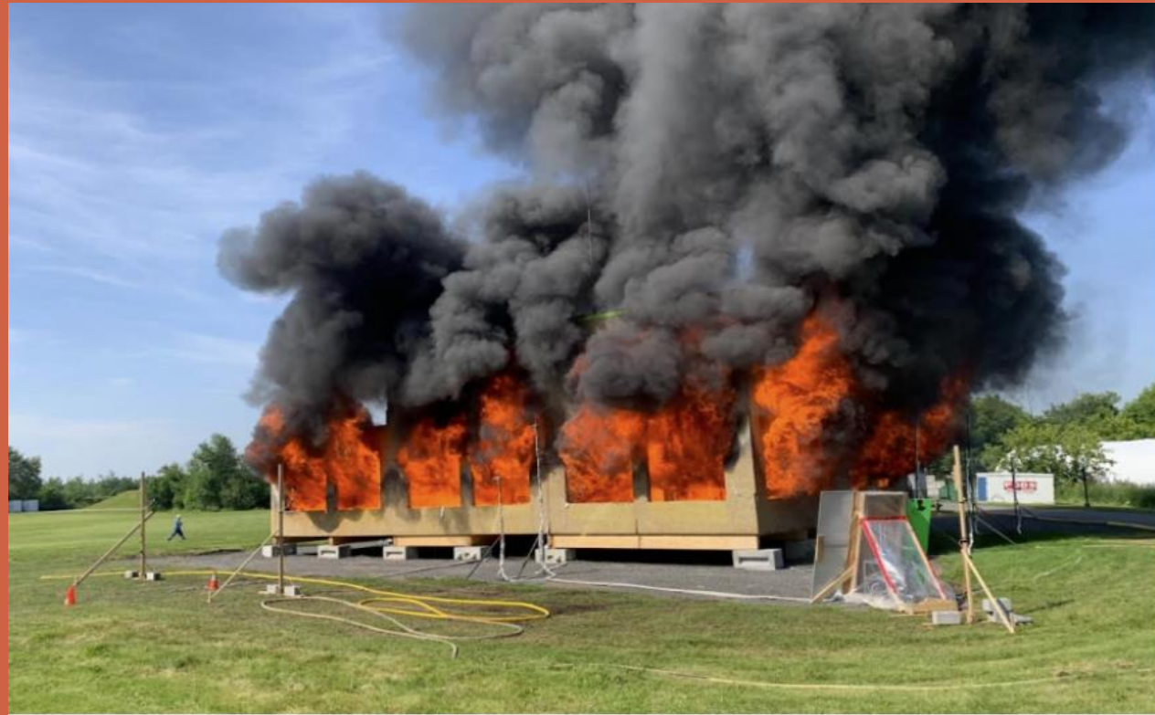
Mass timber structure during the fully developed fire.
