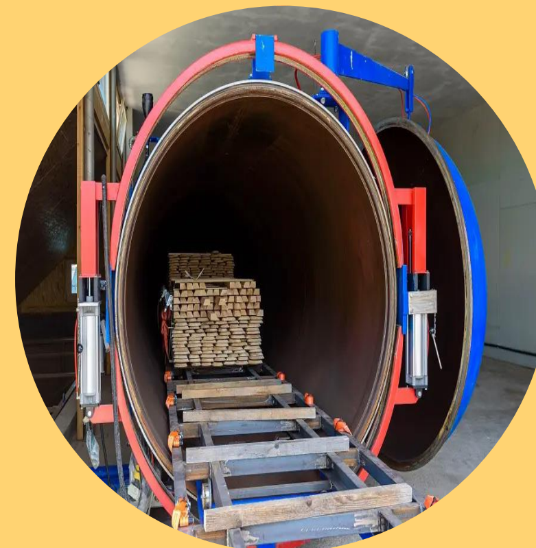
Fire retardant impregnation
